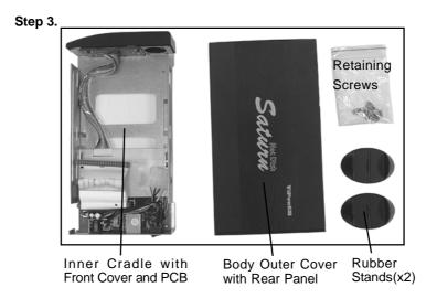
The illustration is the Components of the VPA-3528Net NetWork Storage.
